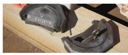
With all preparations complete, the pipe was sheared off. Flow was immediately visible from the bell nipple after closure of the blind/shear rams. The rig tongs were rigged up to a crane, by way of a sheave, and the pipe was rotated to ensure a complete shear was present. The CT equipment and pipe stub were raised above the blinds by the bulldozer and the blinds were closed. All flow was diverted to the flare pit.
